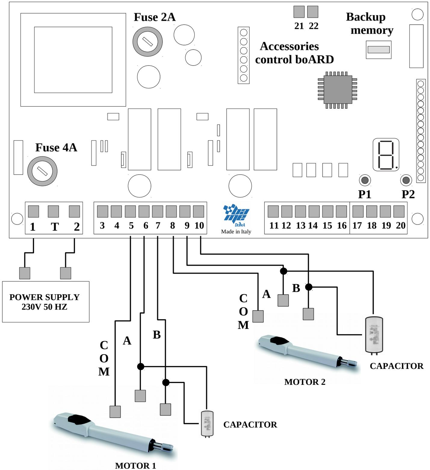
In case the motor start in closing direction, during the first movement on programming, REVERT cable A and cable B
